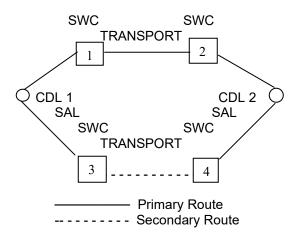
Two diverse circuits between serving wire centers. The SAL and Transport facilities must be entirely separate.
