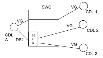
The customer requests that the voiceband circuit (VG) between CDL A and CDL 1 be "rolled over" to the DS1 servingCDL A. No NRCs apply for this request.
