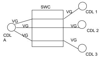
The customer requests the installation of a DS1 between the serving wire center (SWC) and CDL A and a DS1/voice multiplexer in the SWC. The customer also requests that the voiceband circuits serving CDLs 1, 2 and 3 be "rolled over" to the new DS1. All NRCs apply for the installation of the DS1 and multiplexer. No NRCs apply for the voiceband rollovers to the new high capacity circuit.
