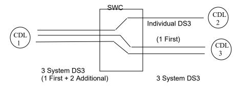
For 3 System DS3s and Unlimited System DS3s ordered under a PBA, each CDL must have a first system SAL. Additional SALs may then be ordered under the normal System terms and conditions.
