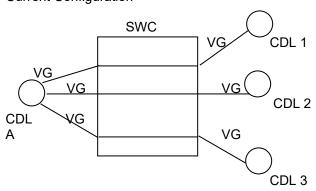
The customer requests the installation of a DS1 between the serving wire center (SWC) and CDL A and a DS1/voice multiplexer in the SWC. The customer also requests that the voiceband circuits serving CDLs 1, 2 and 3 be "rolled over" to the new DS1. All NRCs apply for the installation of the DS1 and multiplexer. No NRCs apply for the voiceband rollovers to the new high capacity circuit.
